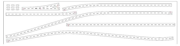
This is a nice, efficient arrangement of the pieces. The bottommost spline was rotated about 160 degrees from its original position to make good use of material. The less material you use, the less you'll pay for your Layout Splines. Make sure to leave at least 1/8" between adjacent splines for the cutting tool.
