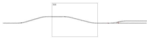
The large box is the size of the material than can be handled by the cutting tool. A set of connectors is in the upper-left of the material box, grouped so they can easily be relocated as a set. We also see the Track Splines that have been built. Note that only the Layout Splines layer is active and displayed. It's easy to toggle **Layout Splines Only** mode: View / Show / **Layout Splines Only** (Ctrl+F12). With the select tool, move the splines into the material box in a compact arrangement.
