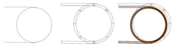
The original track centerlines are shown on the left. The center image shows 3" Roadbed Splines built from the track and the right images shows the track with rails and ties superimposed on the Roadbed Splines. Note now the splines do not overlay the track as one might expect. That's because the very steep grade had to be accounted for when building the splines. Without compensating for grade, the splines would be too short and serve no purpose.
